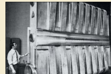
The prototype r.f. cavity, which achieved accelerating field gradients comfortably in excess of design figures.
